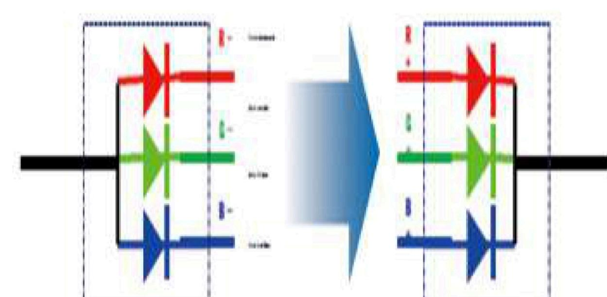
The Common Cathode Solution offers 40% energy savings and reduces temperature by 20°C, ensuring higher efficiency, lower power consumption, and superior heat dissipation for brighter, cooler, and more durable LED displays.
